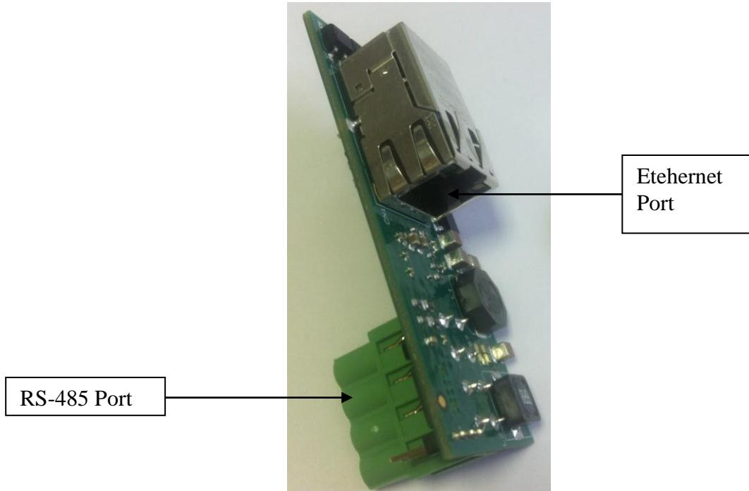
When adding to previously installed barriers, with power already present on the barrier, to make the connection to the Ethernet network use the IP-DOORWAY-C and open links S1, S2, S4, S5.
