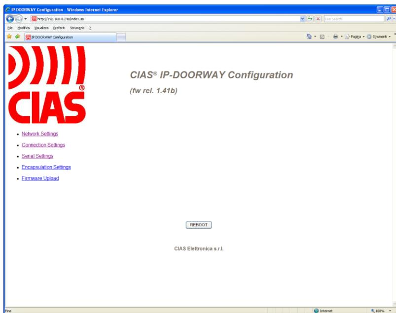
In this section it is possible to modify the IP-DOORWAY parameters:
