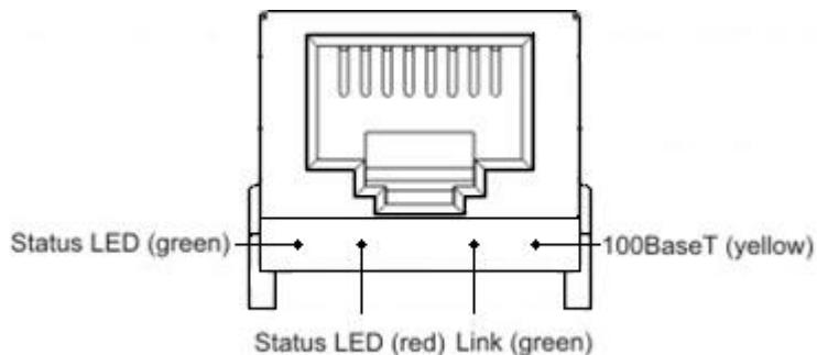
The yellow **100BaseT** led will illuminate if the network supports 100Mb/s data transmission. Install and connect all the IP-DOORWAY that are required on the network.
