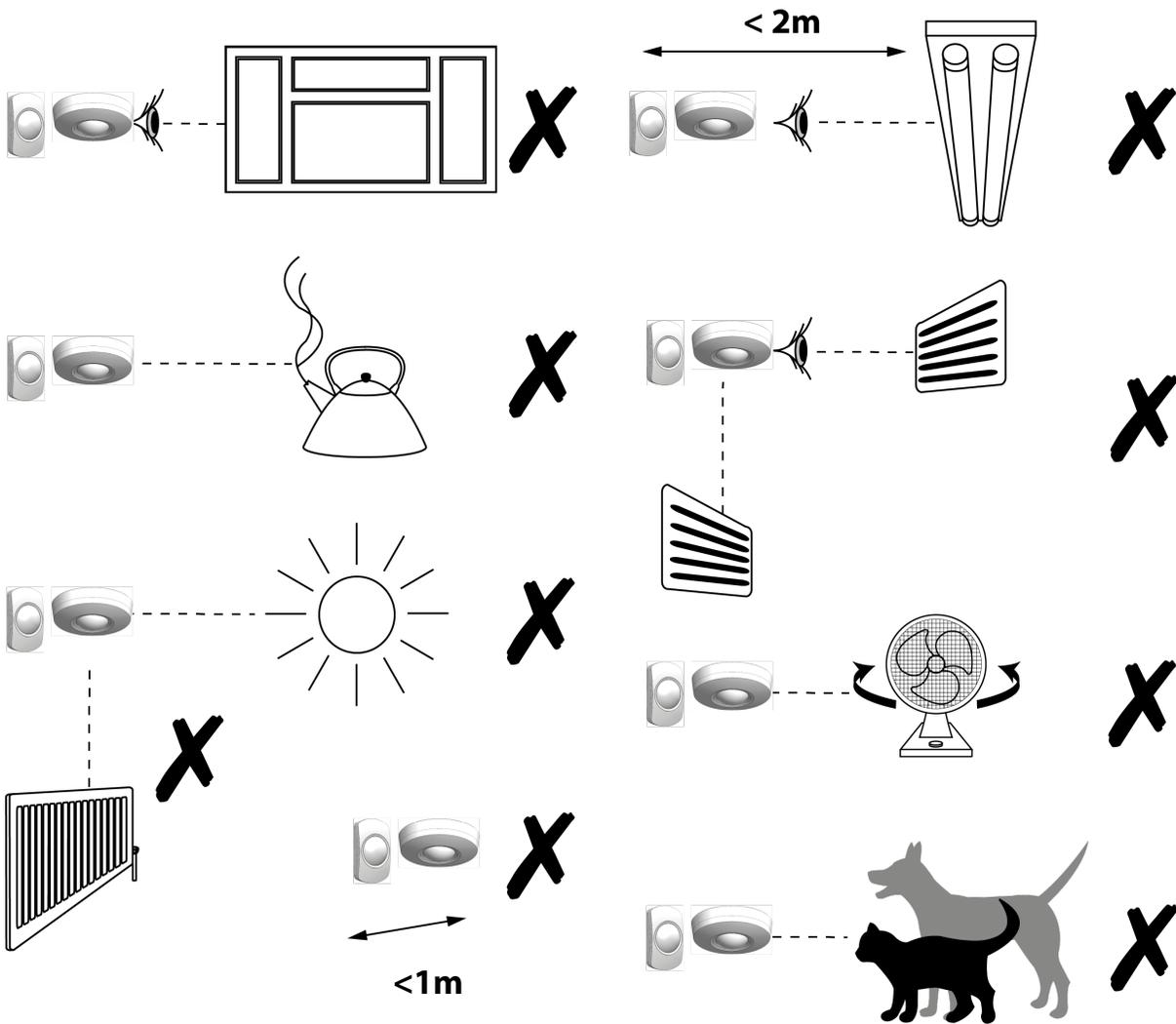
**Ensure the devices field of view is not obstructed**
