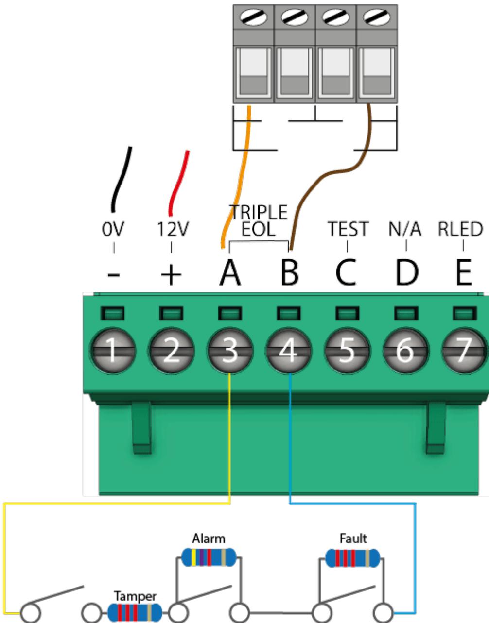
**Fault Monitoring** - A fault will be indicated by one of the following:
